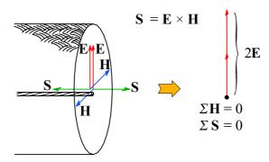
**Fig.8:** Vector sum of the outward and inward reflected components at the open end of the coaxial cable: the electric component **E** doubles, whilst the magnetic component **H** cancels, and so does the Poynting's vector **S**. The result is an apparently static electric field.
