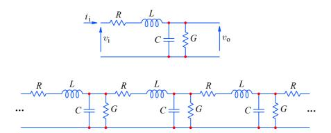
**Fig.3:** Above: Electrical lumped circuit model of a small segment of a coaxial cable. The core has a small serial resistance R and a serial inductance L. Its capacitance to the shield is represented by C and the conductance of the insulating material between the core and the shield is represented by G. **Below:** a long cable can be modeled by an infinite series of such small segments.
