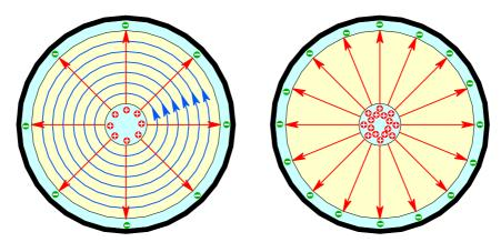
**Fig.A1.1:** Left: Field cross-section under the propagation condition, with the radial electric field and circular magnetic field. **Right:** under the superposition with the reflected wave the magnetic field cancels and the density of the electric field doubles.
