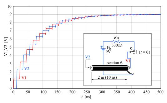
**Fig.9:** Refilling the cable with energy from the battery through a  $330\,\Omega$  resistor. The mismatch of impedance  $Z_0/R_{\rm B}$  and the time delay cause a stairstep like voltage build up. The small aberrations at each transition are the consequence of the oscilloscope input capacitance (~12 pF) loading of the line.
