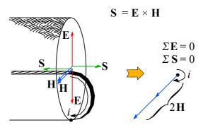
**Fig.9:** Vector sum of the outward and inward reflected components at a shorted end of a coaxial cable. The magnetic component doubles, caused by a loop current i, whilst the electric component cancels, and so is the Poynting's vector. The result is an apparently static magnetic field.
