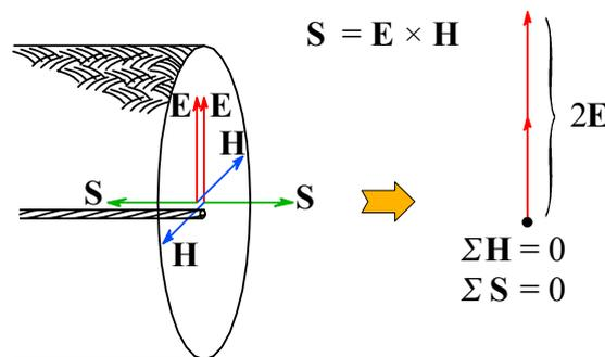
**Fig.8:** Vector sum of the outward and inward reflected components at the open end of the coaxial cable: the electric component **E** doubles, whilst the magnetic component **H** cancels, and so does the Poynting's vector **S**. The result is an apparently static electric field.
