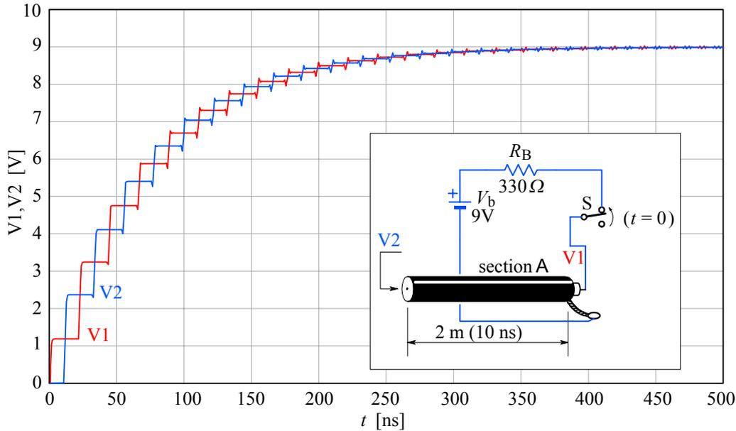
**Fig.9:** Refilling the cable with energy from the battery through a  $330\ \Omega$  resistor. The mismatch of impedance  $Z_0/R_B$  and the time delay cause a staircase like voltage build up. The small aberrations at each transition are the consequence of the oscilloscope input capacitance ( $\sim 12\text{ pF}$ ) loading of the line.
