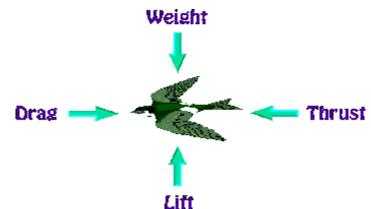
Heavier-than-air flight is made possible by a careful balance of four physical forces: <u>lift</u>, <u>drag</u>, <u>weight</u>, and <u>thrust</u>. For flight, an aircraft's lift must balance its weight, and its thrust must exceed its drag. A plane uses its wings for lift and its engines for thrust. Drag is reduced by a plane's smooth shape and its weight is controlled by the materials it is constructed of.
