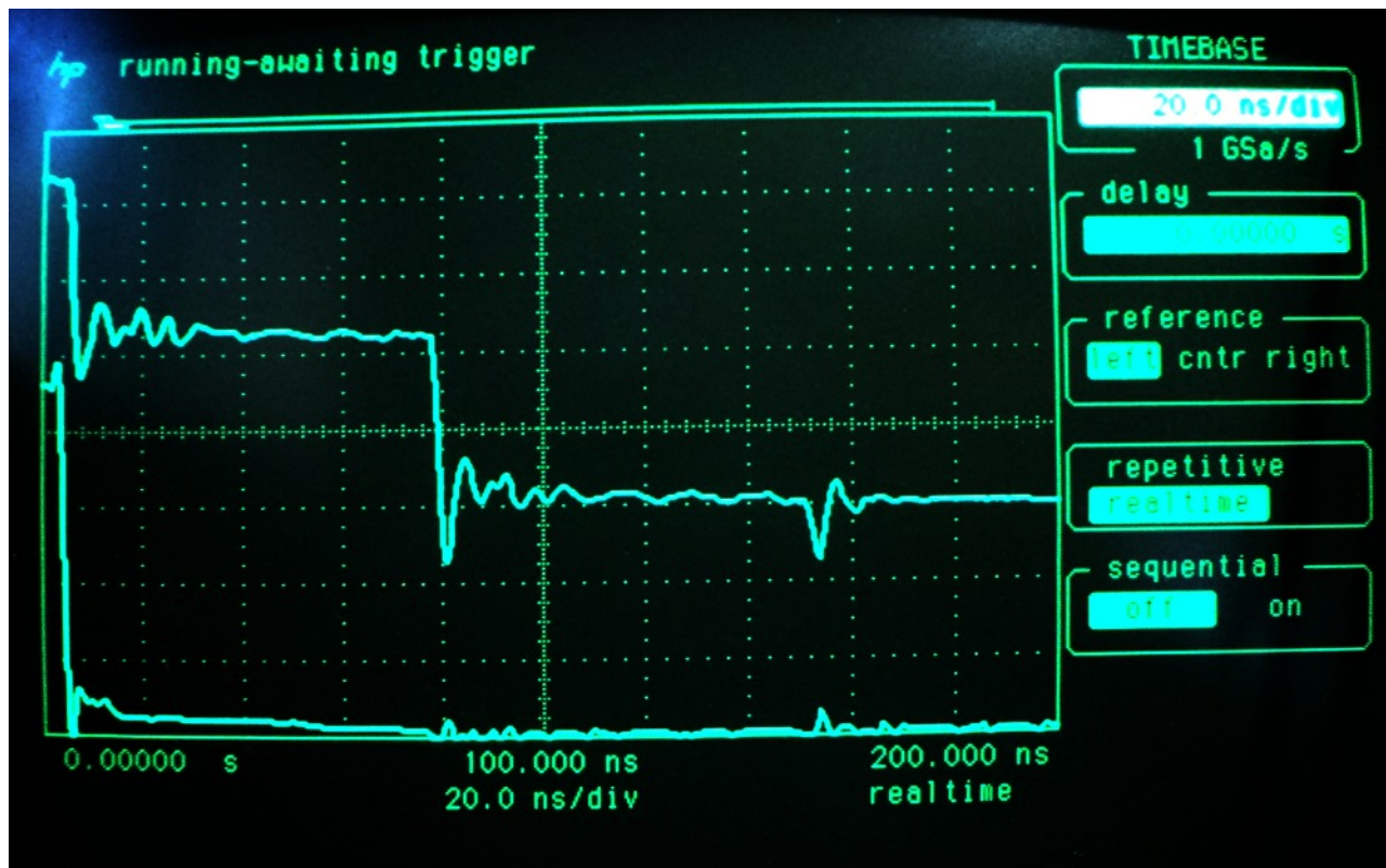
Top Trace Across 75 ohm termination 18 Meters Length of 75 Ohm cable Point 'A'
