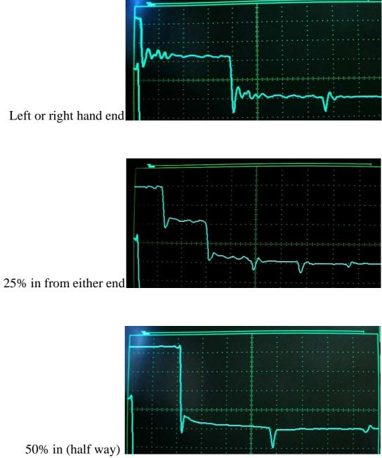
The moment the switches close, there are no more reflections at either end. The energy that was travelling to the right exits on the right, and the energy that was travelling to the left exits on the left. The width of each exiting pulse is now equal to the delay down the charged cable, not double as before.
