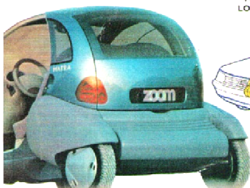
Renault's 75 mph electric ZOOM shrinks to 2.1 m length for parking
