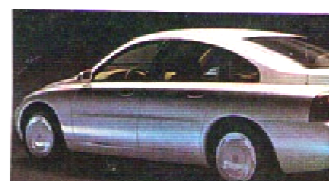
Volvo's 108 mph, four-seater gas-electric ECC hybrid
