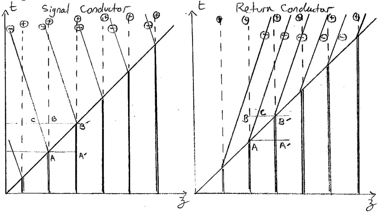
As the wave passes each atom the positive charge remains stationary - for example the lines AB - while the electrons begin to drift - for example from A to C on the diagram. The distance BC is thus  $v \delta t$ . If, as shown,  $\delta t$  is the time for the wave to advance to the next atom, with atomic spacing  $a$ , then  $\delta t = a/c$ .
