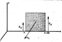
where we are to take the values of  $E_y$  at x+dx and x, respectively. The difference between these two values of  $E_y$  at the two positions is  $(\partial E_y/\partial x)dx$ , so we can write the line integral of Faraday's law of induction as
