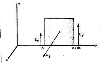
where we are to take the values of  $E_y$  at x + dx and x, respectively. The difference between these two values of  $E_y$  at the two positions is  $(\partial E_y/\partial x)dx$ , so we can write the line integral of Faraday's law of induction as
