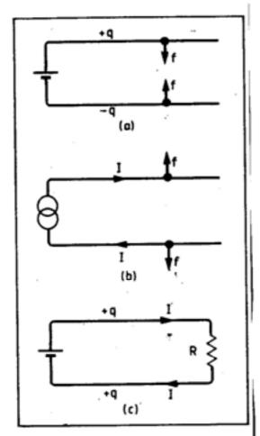
that if a line has Z<sub>0</sub> = 100Ω then to establish a current of 1A in the line we need a supply of 100V and the electrostatic attraction because of that cannot be ignored.
