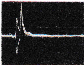
Fig. 42. Same as Fig. 40 but with 120 ohms ( \approx Z_{0c} ) connected between the far ends of the active and the passive line.
