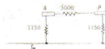
Fig. 43. Same as Fig. 40 but with the two lines terminated in the correct delta of resistors. Vertical scale: uncalibrated. Horizontal scale: 5 ns/div.
