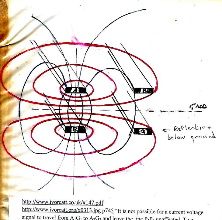
signal to travel from A<sub>1</sub>G<sub>1</sub> to A<sub>2</sub>G<sub>2</sub> and leave the line P<sub>1</sub>P<sub>2</sub> unaffected. Two fundamental TEM modes can exist .... Even Mode .... Odd Mode ...."
