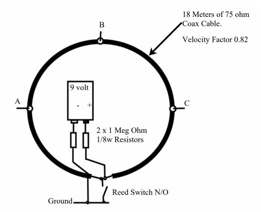
Some may say that we should use two reed switches but as we are only interested in showing what happens after the short is applied to both ends of the Coax we can get away with one switch and joining both ends of coax together.
