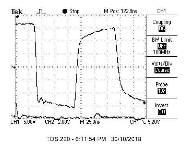
Waveform as seen at point B centre line of display is 0 volts each division in Horizontal direction is 25 ns. Vertical is 2 volts per division.
