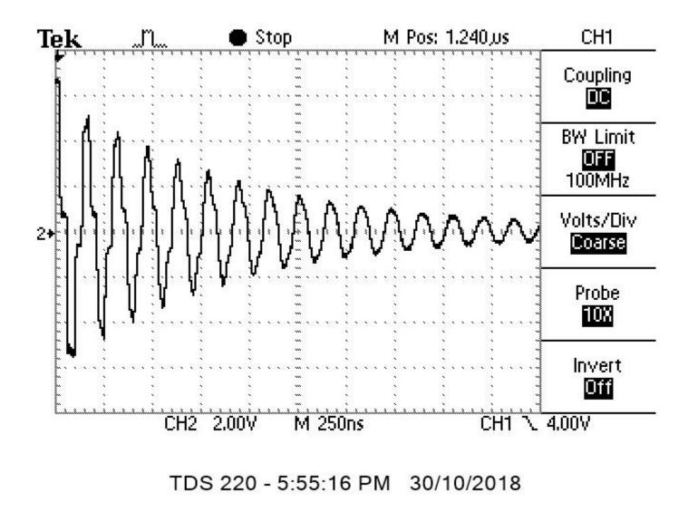
Waveform as seen at point B centre line of display is 0 volts each division in Horizontal direction is 50 ns. Vertical is 2 volts per division.
