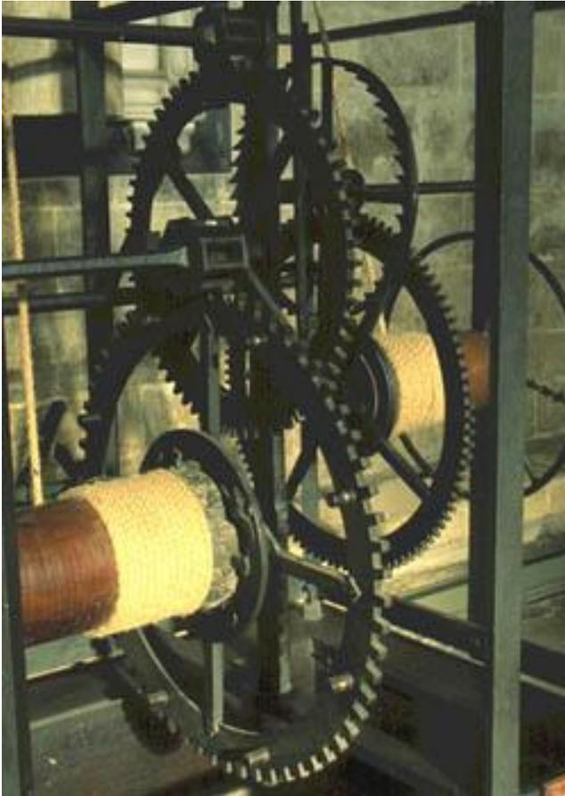
In 1386, the first mechanical clock on record in Britain was installed at Salisbury Cathedral. It has no face and only strikes the hours.
