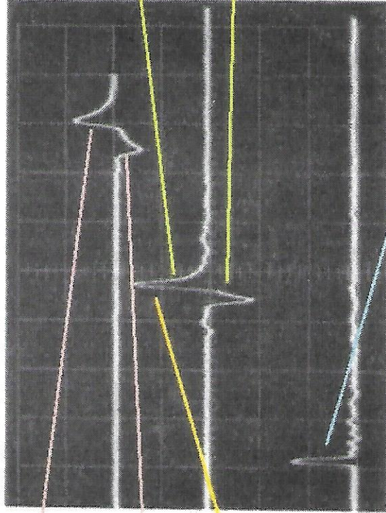
Fig. 29. Passive line. Third trace: front end of line. Second trace: 120 inches down line. First trace: 234 inches down line.
